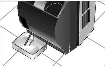
There are castors fitted on your appliance to make moving it easier. If it is necessary to tilt your appliance in order to move it, then the internal water tank must be drained first. To do this, connect drainage pipe to stopcock at the bottom of the appliance.
